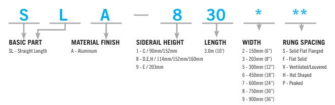
The types of covers that can be ordered are Solid Flat with Flange (S), Flat (F), Ventilated (V), Hat (H), and Peaked (P). Covers can be ordered with indoor or outdoor heavy duty fastening systems. Covers should be installed where there is the possibility of cable damage from falling objects or items being placed on the tray.
